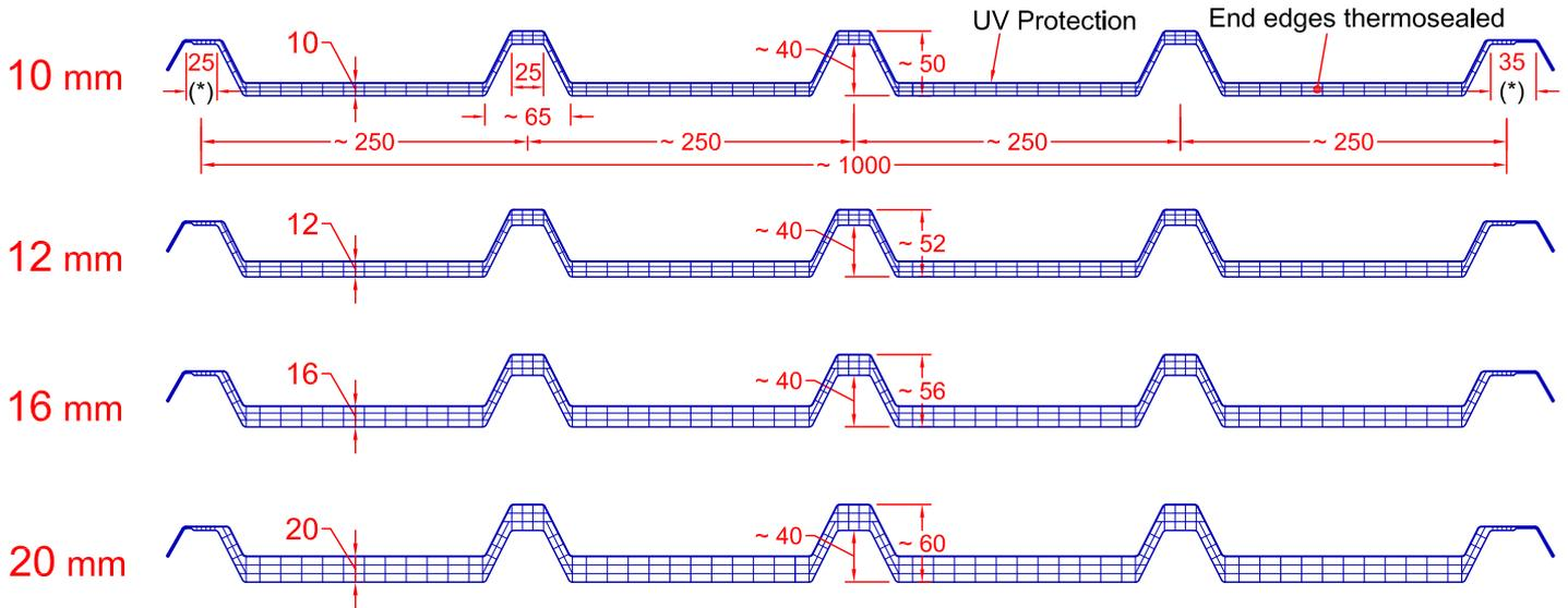
(\*) Standard width of lateral hooks 25 / 35 mm- alterable on request (min 20, max 40 mm)
