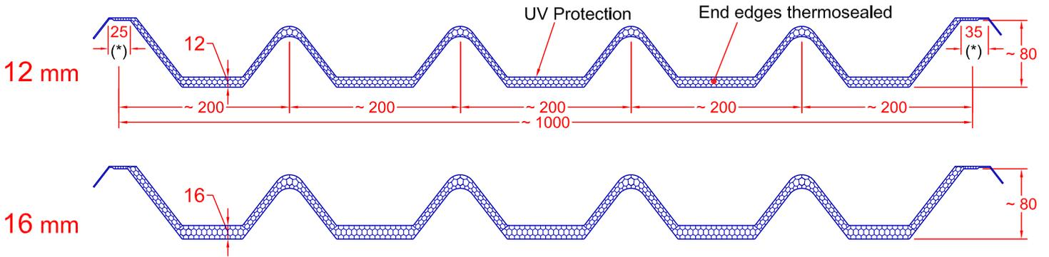
(\*) Standard width of lateral hooks 25 / 35 mm- alterable on request (min 20, max 40 mm)
