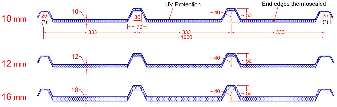
(\*) Standard width of lateral hooks 25 / 35 mm- alterable on request (min 20, max 40 mm)t
